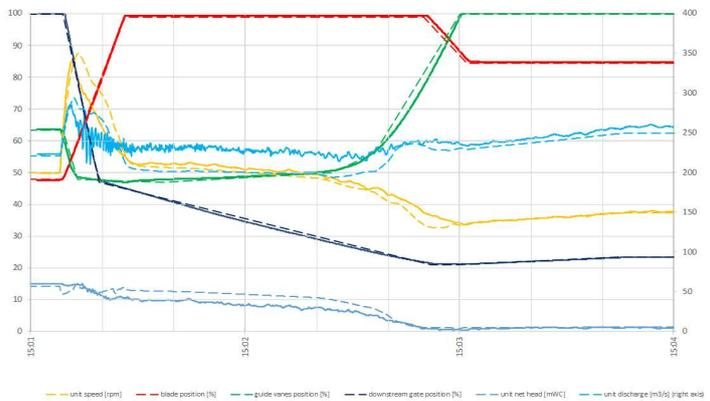
Figure 11: Flow transition from turbine mode to sluicing mode initial discharge 222 m<sup>3</sup>/s, gross head 14.5m. Comparison between measurements (plain lines) and computations (dashed lines)
