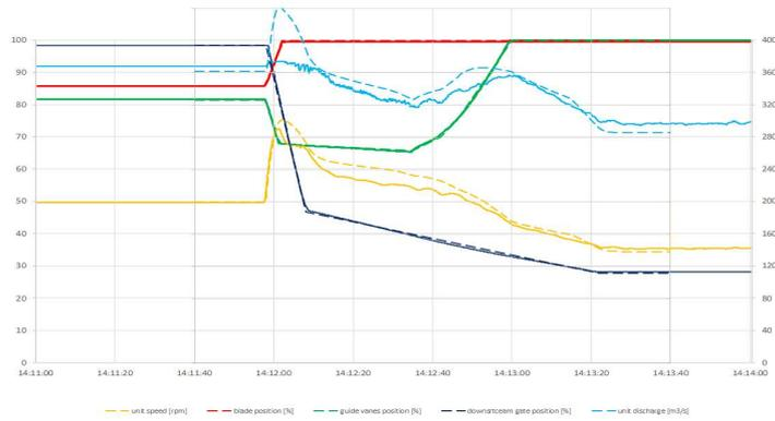
Figure 10: Flow transition from turbine mode to sluicing mode initial discharge 368 m<sup>3</sup>/s, gross head 12.3m. Comparison between measurements (plain lines) and computations (dashed lines)
