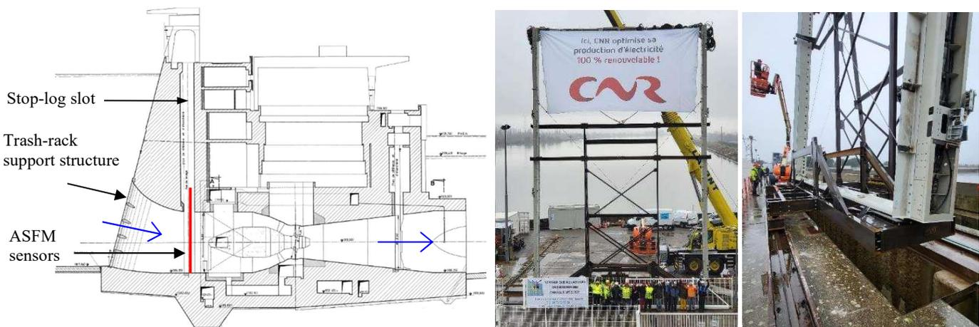
Figure 4: Vertical cross section of Beaucaire intake (left) – Frame positioned onto the trolley (center and right)
