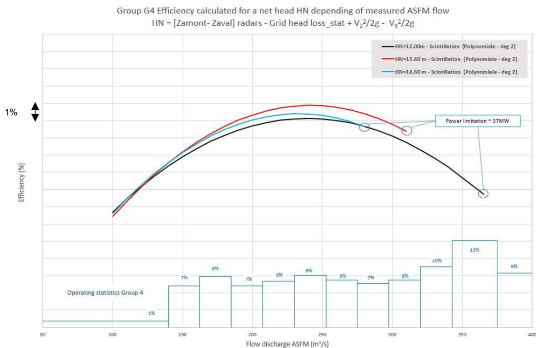
Figure 7: Efficiency results of the Beaucaire campaign for 3 net head: 12m, 13.4 and 14.6m
