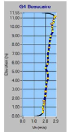
Figure 1: Results of computed velocity,  $Q=284.47\text{m}^3/\text{s}$
