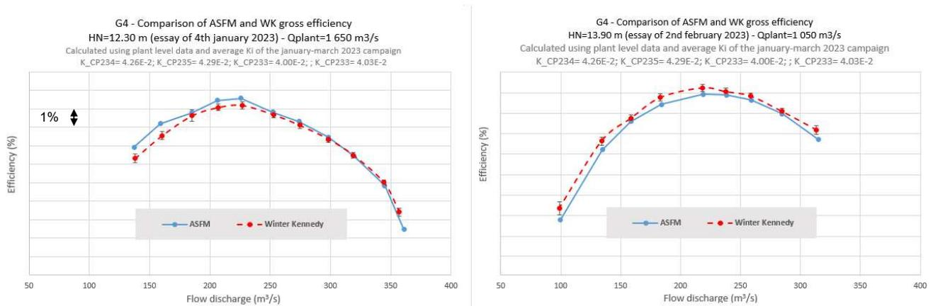
Figure 8: Comparison of efficiency with WK and ASFM results
