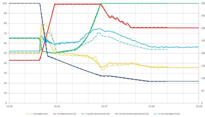
Figure 9: Flow transition from turbine mode to sluicing mode initial discharge 210 m<sup>3</sup>/s, gross head 12.2m. Comparison between measurements (plain lines) and computations (dashed lines)
