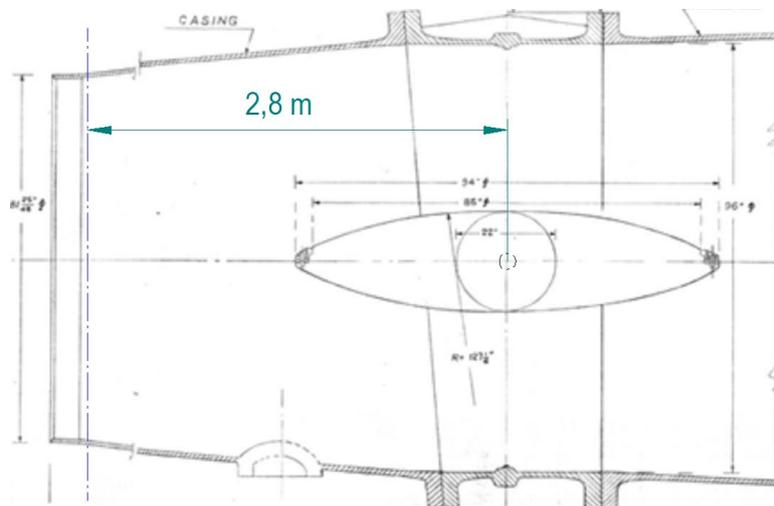
Figure 6 Location of the valve body to the measuring section
