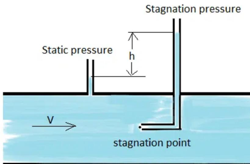
Figure 1: Sketch of the Pitot principle:  $h$  is directly proportional to the stagnation pressure and thus directly proportional to the square of the fluid's velocity  $v$ .
