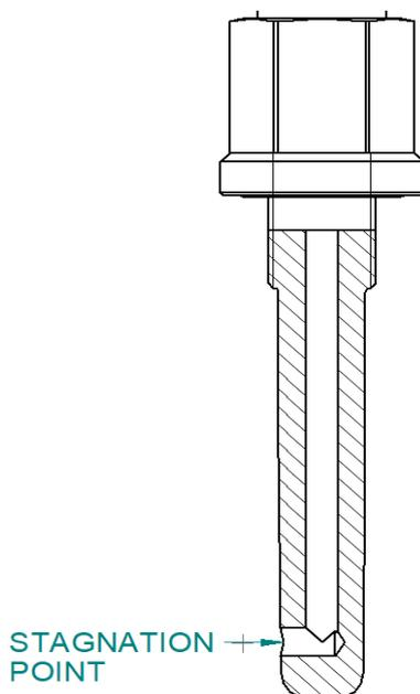
Figure 2 typical design of a sampling probe for thermodynamic test
