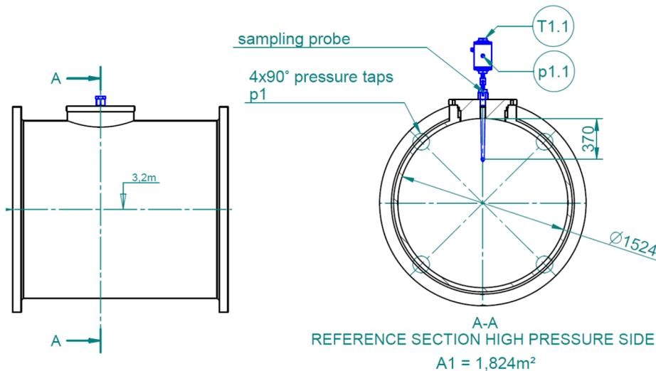
Figure 9 Sampling probe and static pressure taps location
