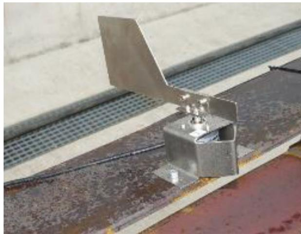
**Figure 8 Angle sensor at measuring frame**
