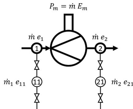
**Figure 2:** thermodynamic system of a turbine with sample extraction into measurement vessels at the reference sections.
