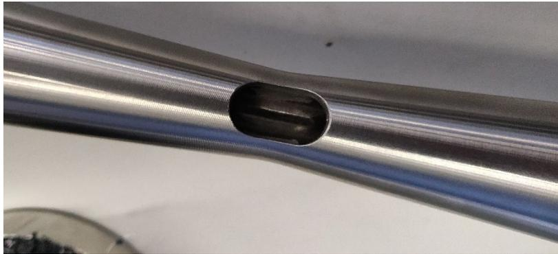
**Figure 7:** Dissipation of inner energy at the extraction of the secondary flow is significantly reduced after enlarging the probe's orifice into a slotted hole and smoothing out the edges on the outer and inner surfaces.
