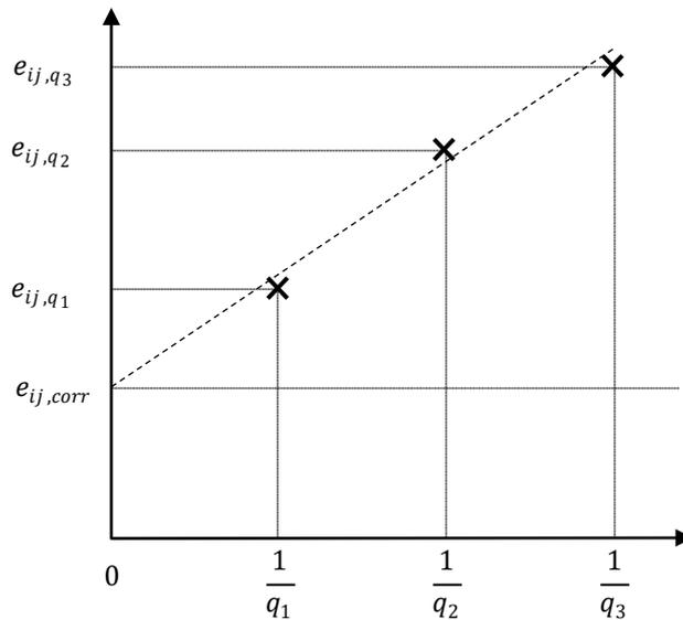
**Figure 3:** Graphical method for correcting the specific energy  $e_{ij}$  for parasitical heat flow as proposed by IEC 60041.
