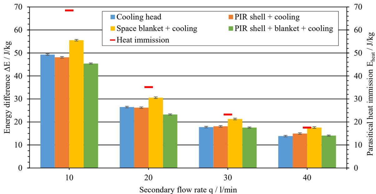
**Figure 6:** Comparison of difference of specific energy of different insulation setups with cooling head on the left ordinate. On the right ordinate with the same scaling is given the parasitical heat flow to the reference vessel.
