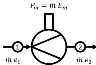
**Figure 1:** A hydropower turbine as thermodynamic system
