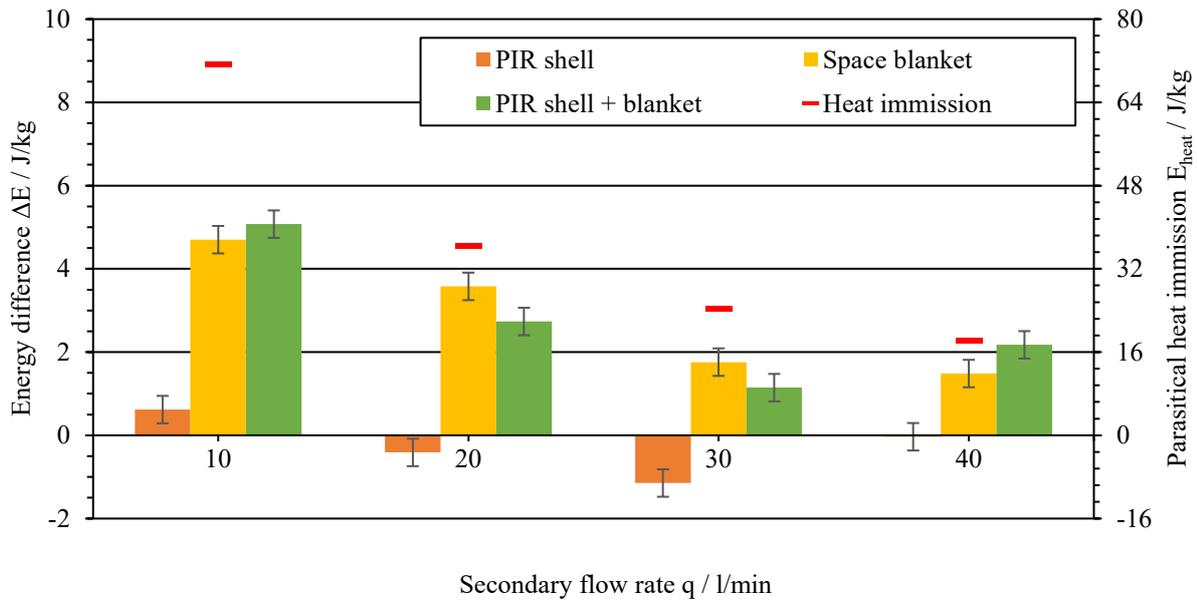
**Figure 5:** Comparison of insulation setups without a cooling head. Given is the difference in measured specific energy between reference and measurement vessel on the left ordinate, and the parasitical heat flow to the reference vessel on the right ordinate. Note that the scaling differs between the ordinates by a factor of 8!
