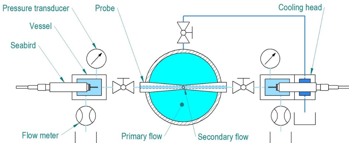
Figure 4: Schematic view of the measurement setup with hydraulic network and section view of the main conduit and shared probe for comparative testing. Left is the reference vessel and right the test vessel shown with cooling head.
