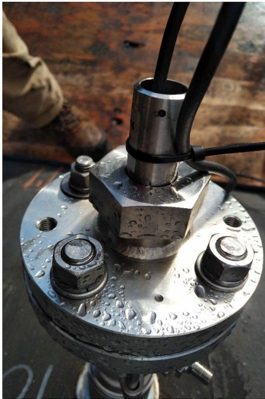
**Figure 3: Acoustic Instrument Installed Through the Valve.**
