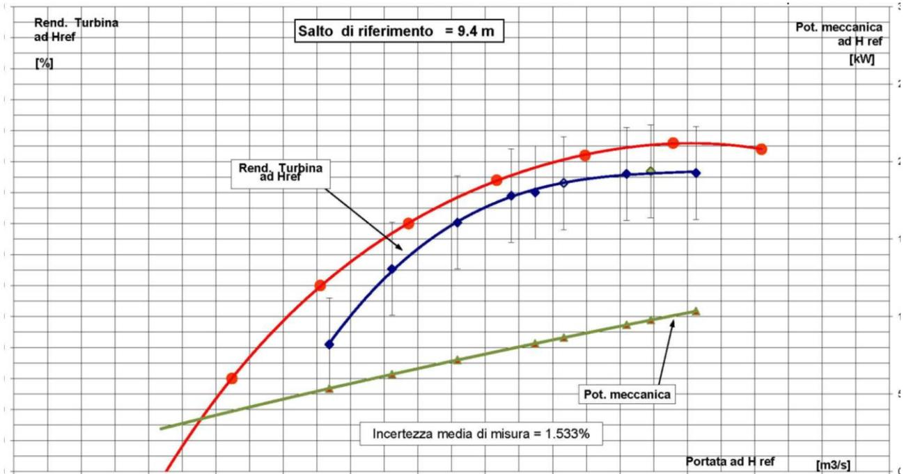
A detailed examination of the measurement errors led on average to an overall error (which takes into account both the systematic and random components) of approximately  $\pm 1.53\%$ .
