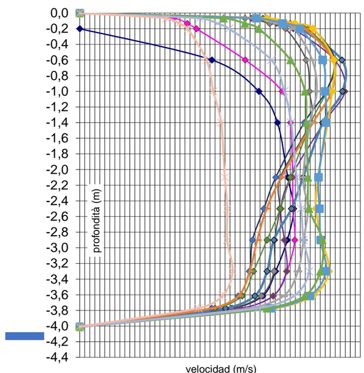
The graphs in the figure represent the speed profiles at the maximum efficiency load of the unit, from which a certain homogeneity of the velocity as the sinking varies can be deduced. Also in this case it was deemed appropriate to use self-component current meters up to angles of  $\pm 45^\circ$ . No recirculations were detected.
