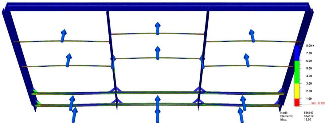
Further fluid dynamic analyses, however, highlighted that in full load conditions in the upper area of the left mouth a localized speed of 5.4 m/s would have been reached, therefore a precautionary evaluation with safety margin of 1.5 has been used. The final FEM analysis of the structure has been performed by considering an homogeneous axial force based on 8.0 m/s flow velocity.
