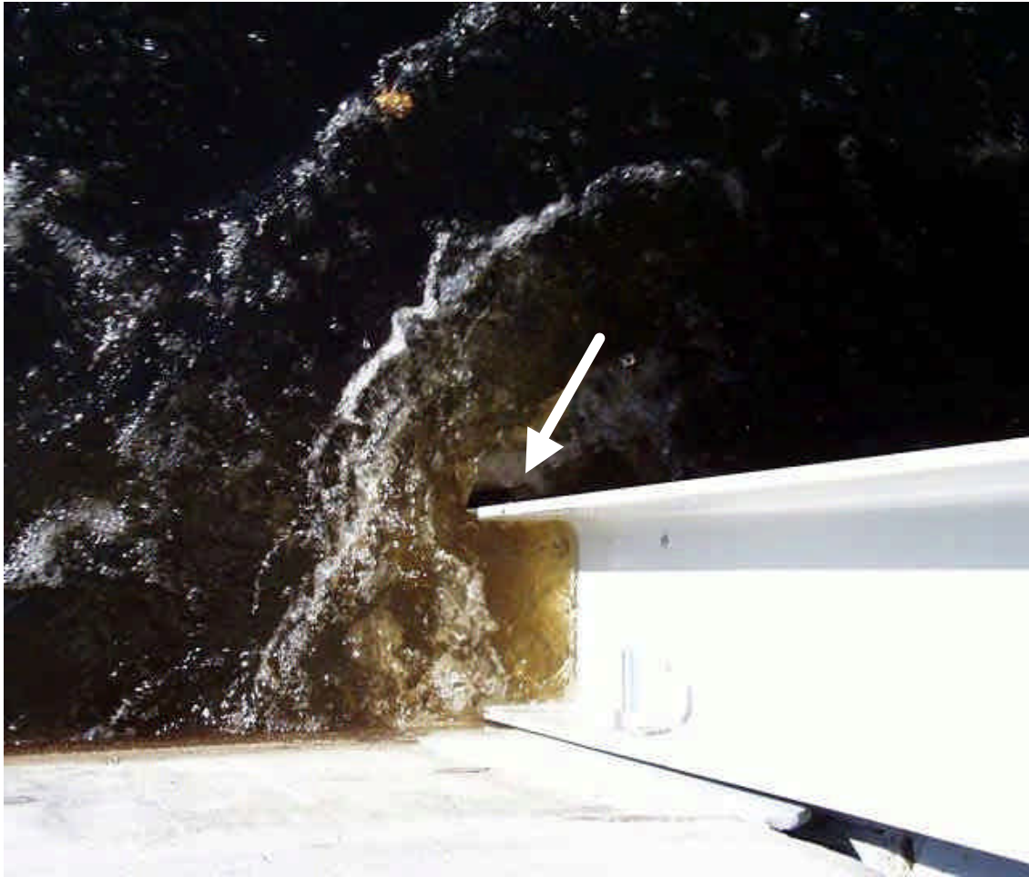
Figure 2-6: Entrainment of air around frame during vibration testing (indicated by white arrow).
