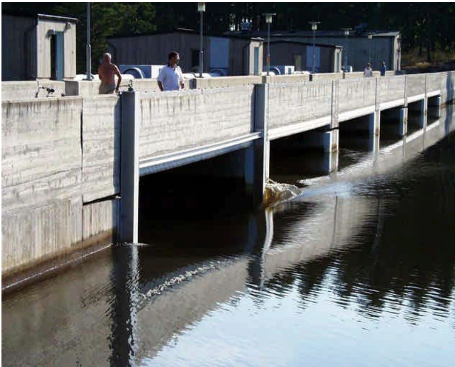
Figure 2-5: Flow through spillway opening during vibration testing (no fairings present).
