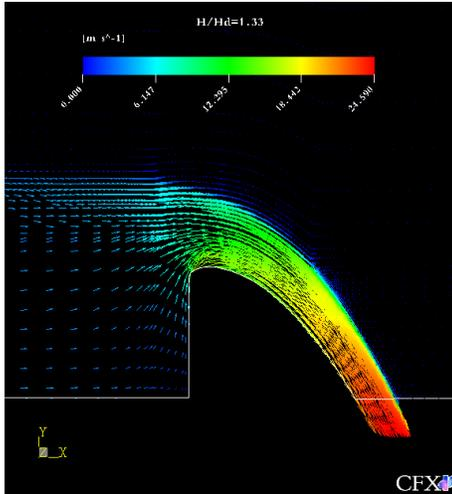
Figure 6:  $H/H_d = 1.33$  2D case. Velocity Vectors.
