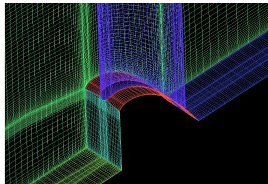
Figure 3: Topology and Mesh of the 3D Ogee Spillway with type 2 Piers.
