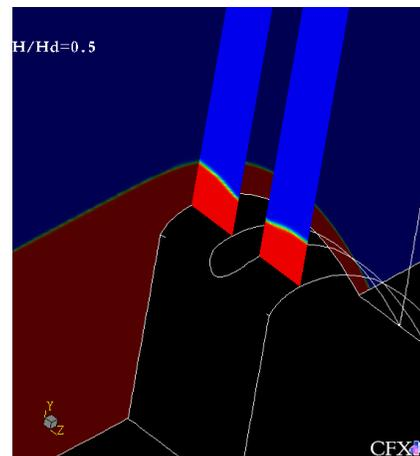
Figure 8:  $H/H_d = 0.5$  3D case. Water Volume Fraction at the center of bay, along piers and at the crest cross section. The red color corresponds to a water volume fraction equal to 1 (water), the blue color corresponds to a water volume fraction equal to 0 (air).
