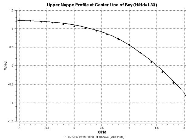
Figure 11:  $H/H_d = 1$  3D case. Pressure field at selected planes (top). Comparison of the Upper Nappe Profiles with USACE data at the center line of bay (middle) and along the pier (bottom).
