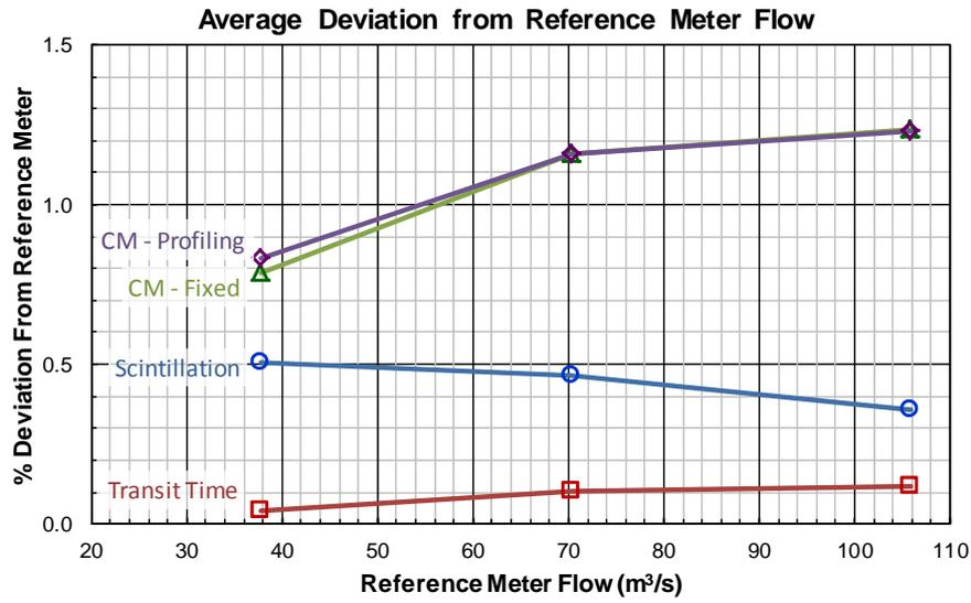
Figure 7 Average Deviation from Reference Meter Flowrate
