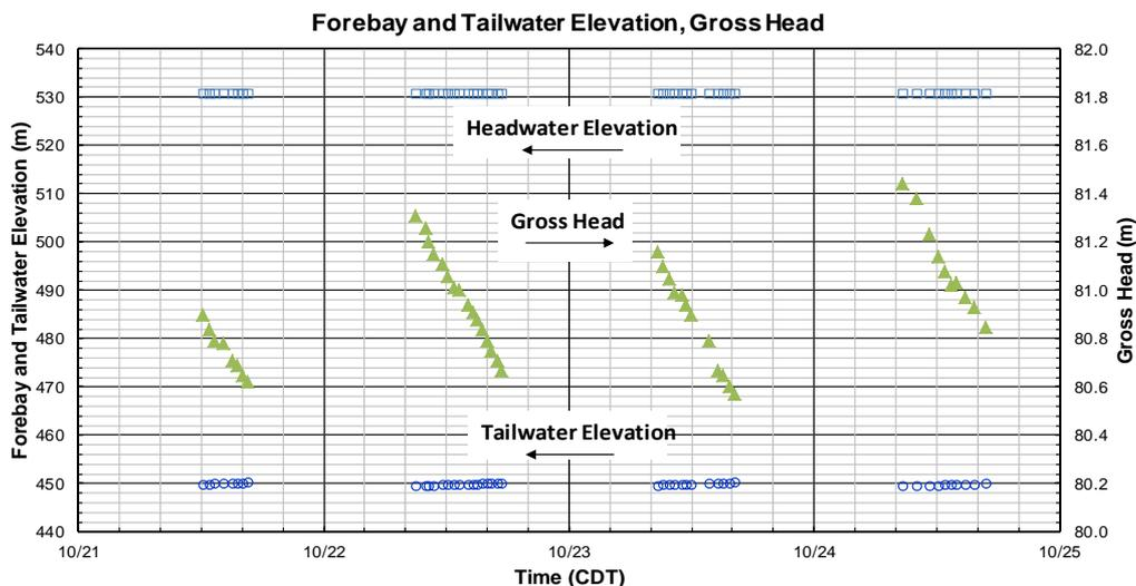
Figure 5 Variation in Head During the Test Program
