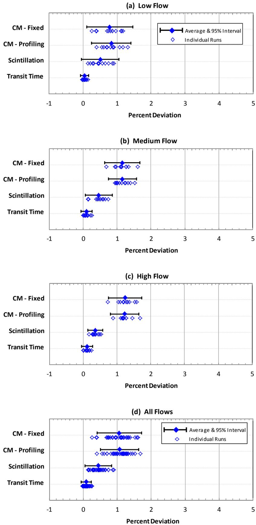
Figures 6(a) – 6(d) Plot of results relative to reference flowmeter
