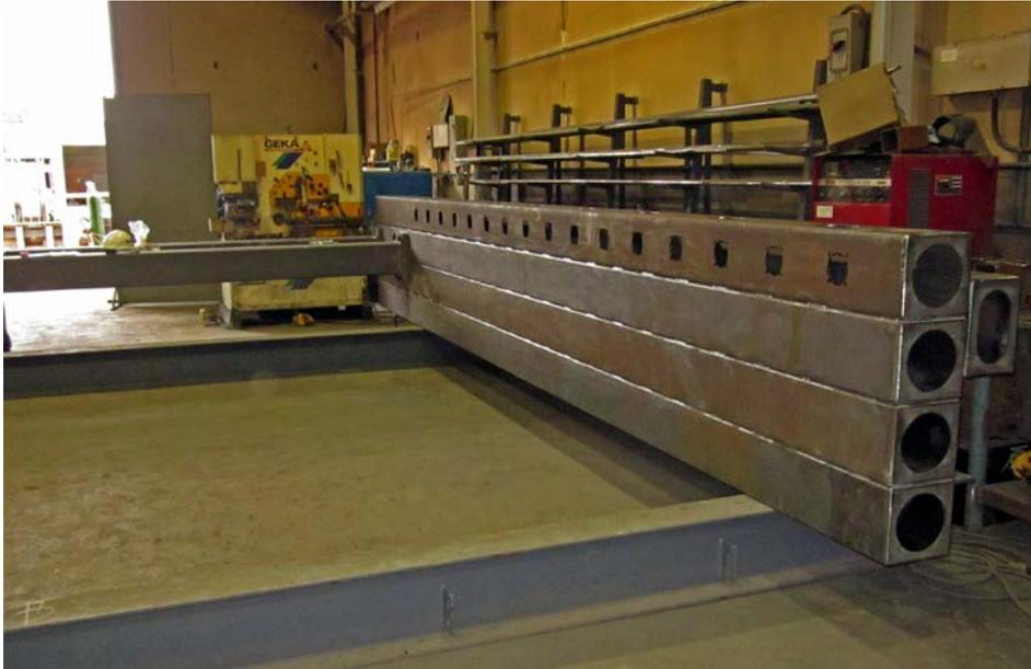
Figure 4 – One side of the AS frame (cross beams holding the two sides together at the top)
