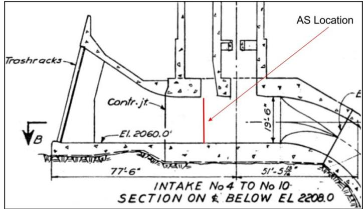
Figure 3: Plan and vertical section of the Unit 4 intake.
