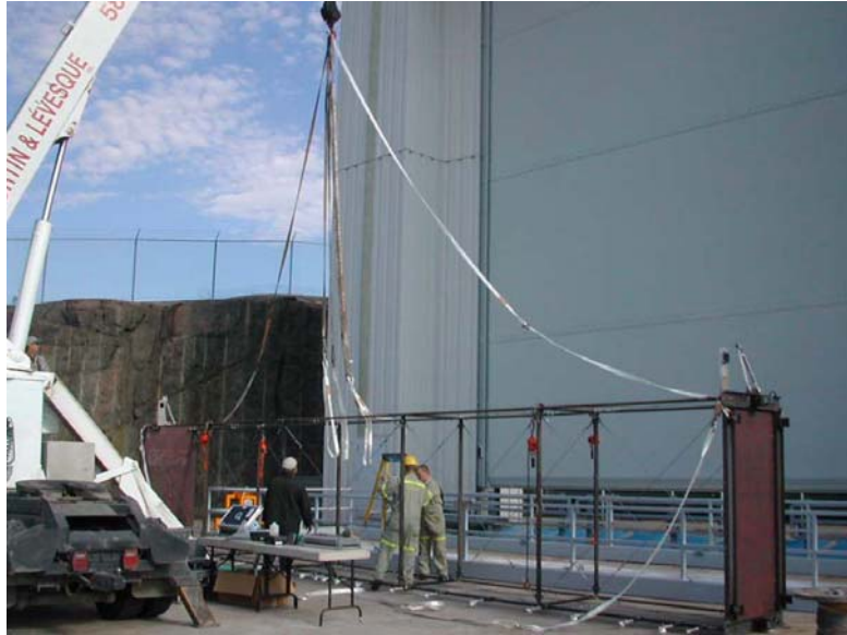
Figure 5. Trolley supporting the Current Meters at Power Plant A
