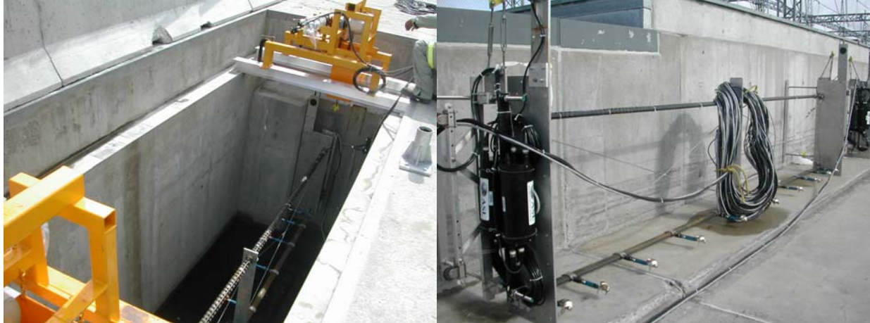
Figure 2. Frame supporting the Acoustic Scintillation transducers and current meters trolley (right) and chain hoists (left).
