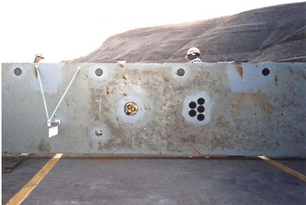
Figure 1: Five arrays in a cluster (right centre). The regular ASFM transducers are along the top of the frame (the downstream edge when the frame is deployed vertically in the intake during measurement); the other instruments visible were used for boundary layer measurements
