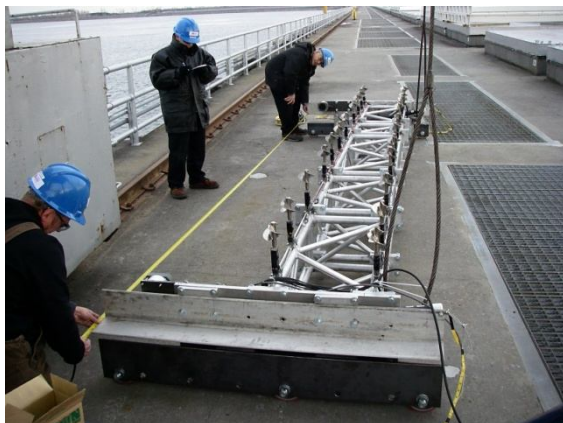
Figure 4: Current meter support frame with ASFM transducer array mounts.
