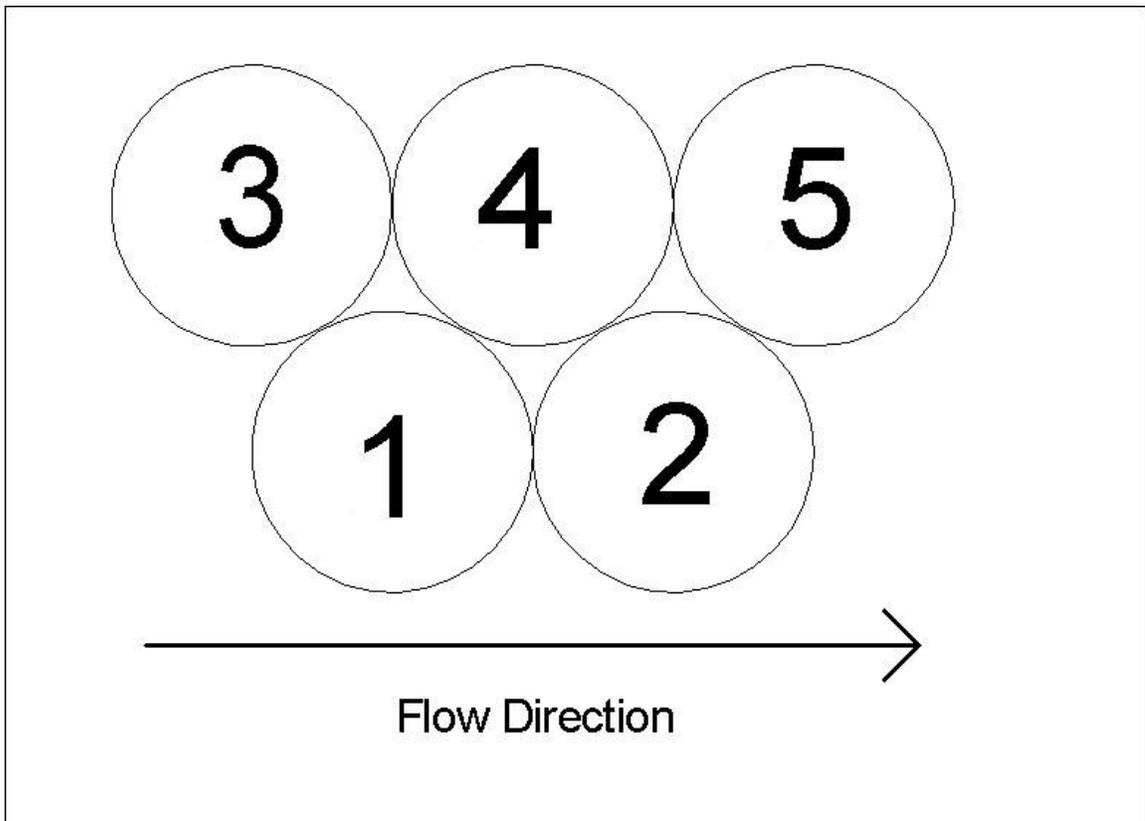
**Figure 4. Schematic representation of the positioning of acoustic transmitter/receiver units in the Lower Monumental Dam studies. The labelling identifies each of the 5 separate measurement lines discussed in the text. In each of these lines, identical arrays were positioned in horizontally-opposing positions at a common vertical level. An equilateral triangular array of transducers as indicated in Figure 1 was contained within each indicated, approximately 10 cm diameter, unit.**
