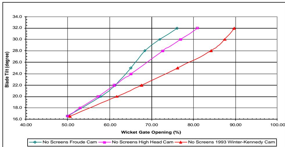
Figure 1: No screens predicted cam curve comparison.
